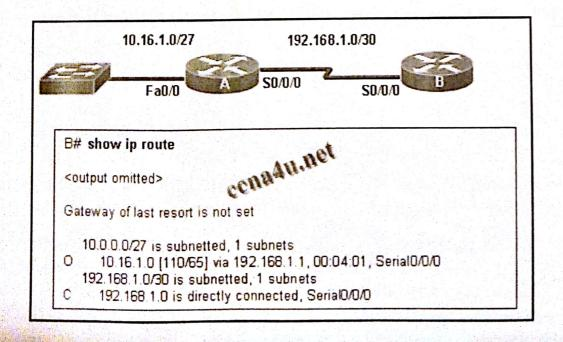
5-Refer to the exhibit. Router A is correctly configured for OSPF. Which OSPF configuration statement or set of statements was entered for router B to generate the exhibited routing table?
