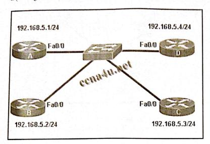
6-Refer to the exhibit. Routers A, B, C, and D are all running OSPF with default router IDs and OSPF interface priorities. Loopback interfaces are not configured and all interfaces are operational. Router D is the DR and router C is the BDR. What happens immediately after the following commands are entered on router A?
